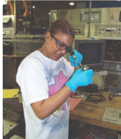
General Automotive Manufacturing's shopfloor personnel spot burrs and other part defects with Hawkeye Precision borescope systems.
