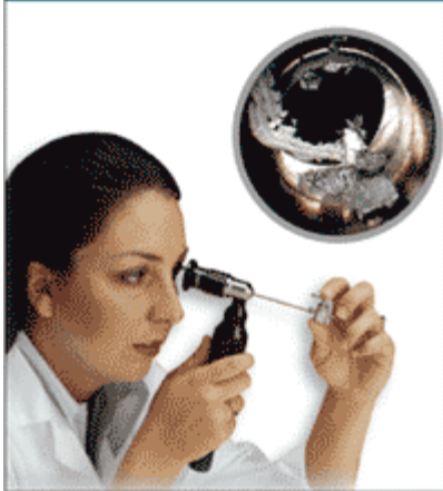
Figure 4: Viewing Chips Inside a Miniature Precision Valve
