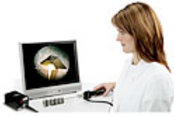
This borescope image is of a spool, made by EDM, used in a hydraulic system for aircraft ailerons. Source: Gradient Lens Corp.
