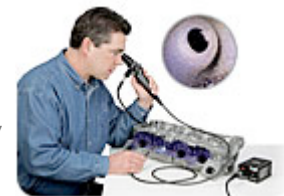
Inspecting a casting, a flexible borescope checks for issues such as porosity or sand. In this instance, an obvious surface anomaly, a burr, is visible. Source: Gradient Lens Corp.
