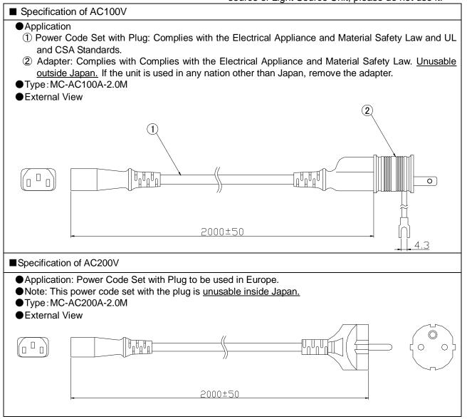
\* The user has to provide an appropriate power supply cord set, conforming to the relevant EU Directives / EN standards with following configurations:
