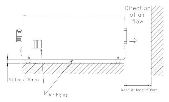
%Horizontal installation with the rubber feet of the unit at the bottom
