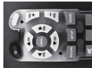
Silkscreen Printing Verification for Remote Control
