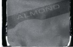
With an IR direct ring LED (MDRL-CIR31)
